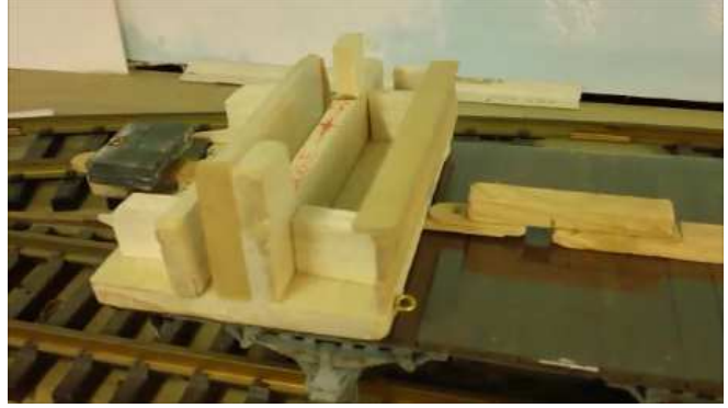
Push Bar rests on an Acetate sheet to slide freely.
