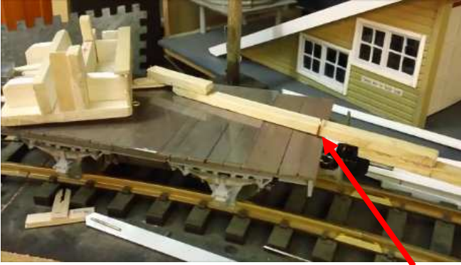
Extended Push Bar 'pivots' in the copper "U" clip.
