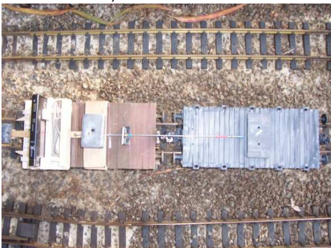
On straight track, the Activation bar has centered the camera ready for a left hand curve Oversteer. This arrangement was not as successful as the bogie wagon versions.
