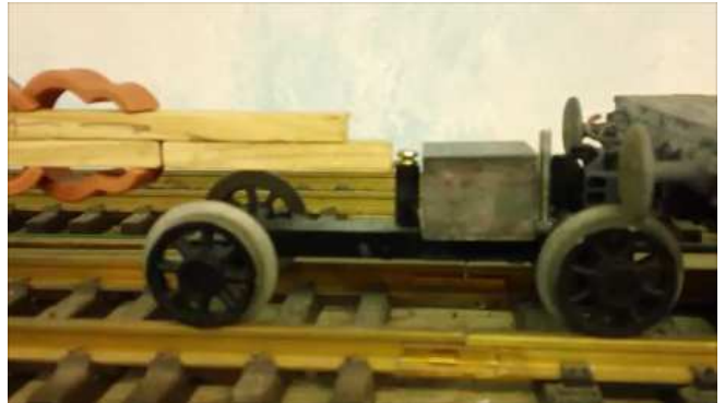
The 'idler' bogie pivot at rear end of Push Bar.
